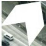
This arrow, which appears when three or more GPS satellites are detected, points in the direction of home. The arrow has eight positions (with 45 degrees between each), and the degrees to the home location is shown below the arrow. (The value is received from the drone's telemetry).
