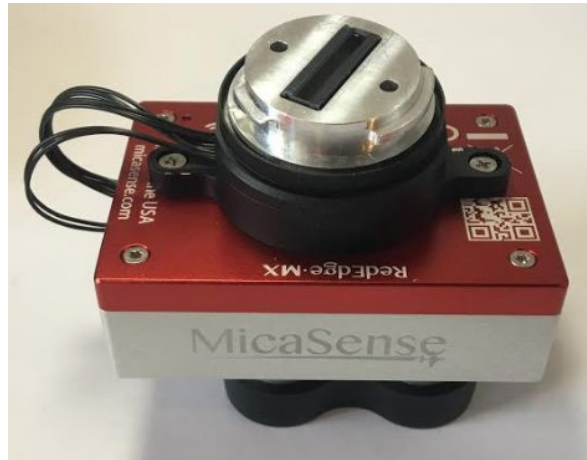
Quick Mount Gen 2 Adapter attached to RedEdge-MX
