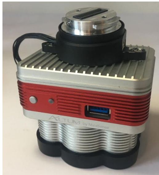
MicaSense Altum connected to Quick Mount Gen. 2
