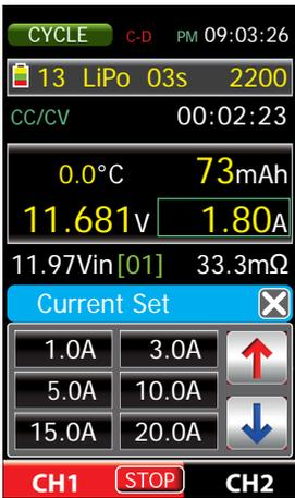
Increase or decrease now by using the INC / DEC buttons to select the current value, such as 1.80 A. If necessary, you can also specify a value that strongly deviate from the current value by touching one of the six option buttons. Tapping the
