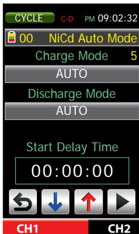
Then you have about five seconds to change the material transferred from the menus “CHARGE” or “DISCHARGE” and charge and discharge mode and, if necessary, set a start delay.
