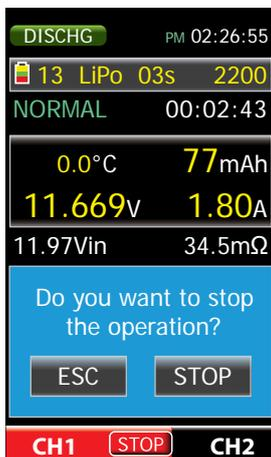
If it is touched the STOP button at the bottom of the display during the actual discharge process, it appears the display on the left. Tapping “Yes“ will cancel the further running in the background discharge. Tapping “No“, the window hides again, and takes the discharge operation run unaffectedly.
