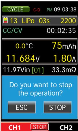
If it is touched the STOP button at the bottom of the display during the actual charge or discharge process, it appears the display on the left. Tapping „Yes“ will cancel the further running in the background. Tapping „No“, the window hides again, and takes the operation run unaffectedly.
