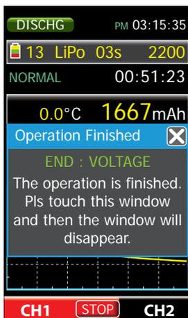
After proper completion of the discharge process the charger emits audible signals and the display shows corresponding informations. So tap the window and afterwards, if necessary, the STOP or ESC key to reverse to basic display.
