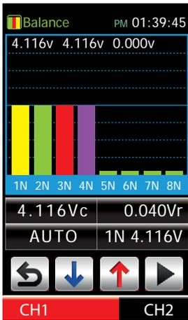
Once the bars are at the same height both in the icon on the top left and in the graphic, the process is complete.
