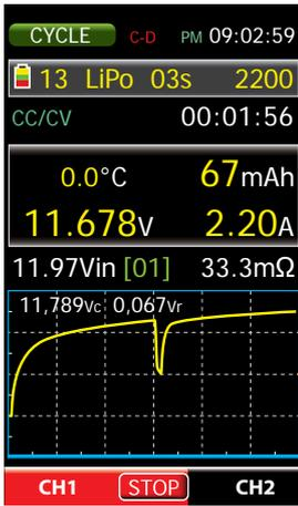
After the lapse of the aforementioned 5 seconds or if necessary, after a manual start, cycle process is begun. Otherwise, an error message is shown.
