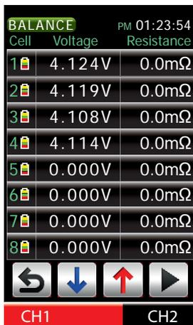
In the second screen of the “BALANCE” menu is shown the current voltage of each individual cell of the battery packs connected to the CH1 or CH2 balancer, maximum of eight cells.
