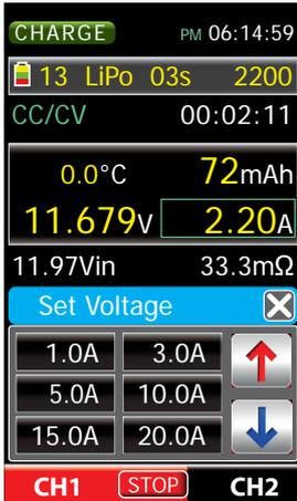
To change the actual charge current tap the display to the actual charge current (6). In the lower half of the display appears a selection window.
