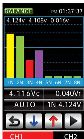
In this third display of “BALANCE” menu are shown graphically, the actual cell voltages of the battery packs connected to the CH1 and CH2 balancer.
