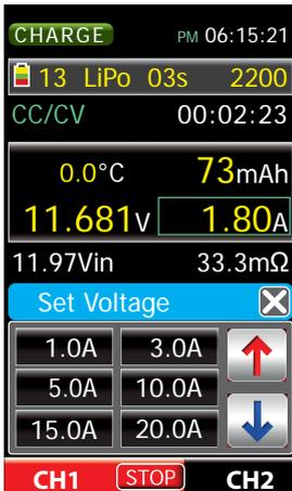
Increase or decrease now by using the INC / DEC buttons to select the current value, such as 1.80 A. If necessary, you can also specify a value that strongly deviate from the current value by touching one of the six option buttons.
