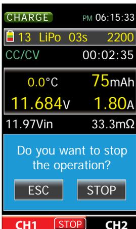
If it is touched the STOP button at the bottom of the display during the actual charge process, it appears the display on the left.
