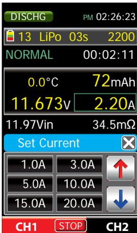
To change the actual discharge current tap the display to the actual discharge current (6). In the lower half of the display appears a selection window.
