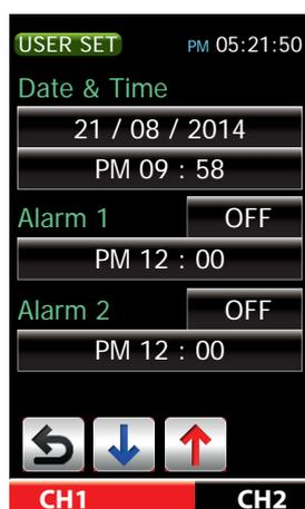
This screen is used to set the date and time \*, and possibly two alarms. After tapping the value to change, this can be changed with the INC / DEC buttons located at the bottom of the display. Tapping again the value field stores the changed value and deactivates the input field again.
