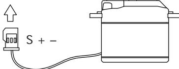
The “servo test” function of this submenu automatically moves the servo connected to the side “SERVO TEST” connector as if, for example, the switch of a transmitter moved continuously and permanently within the set time between its two end points.
