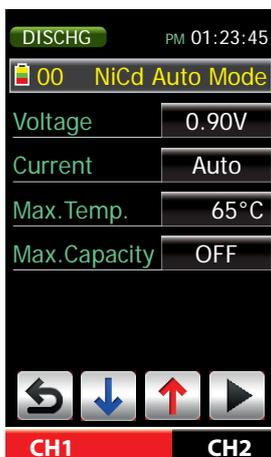
The data concerning your batteries stored in menu "PROFILE" can be added in this menu "DISCHARGE" with the corresponding discharge parameters.
