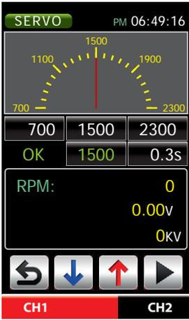
Turn afterwards continuously by hand the shaft of the motor for about 5 seconds. Once the sensor is detected and is fine too, appears OK on the left of the screen instead of the four points. Now you can check the functionality of your controller / motor combination as needed using the servo test function. In order to check the motor speed and power, as shown in the figure below, you need the optional splitter, Order Nr. S8002 grind between motor, controller and charger.
