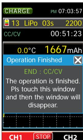
After proper completion of the charge process the charger emits audible signals and the display shows corresponding informations.
