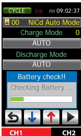
After the expiration of the aforementioned 5 seconds within which you should have at least made the choice of a particular cycle mode as well as the input of a delayed start, it starts an automatic battery test.
