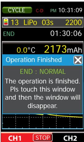
After proper completion of the process the charger emits audible signals and the display shows corresponding informations. So Tap the window and afterwards, if necessary, the STOP or ESC key to reverse to basic display.
