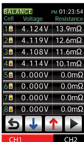
If the battery has already been charged or discharged or at least if it has been previously started a display of the internal resistance, for every single cell it will be shown the internal resistance previously measured in the second page of the menu “BALANCE”, on the right near the individual cell voltage.
