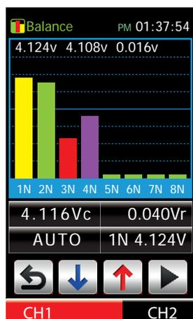
The labeling of the display changes to “Balance” and the height of the bars begins to align gradually.
