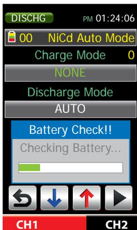
After the expiration of the aforementioned 5 seconds within which you should have at least made the choice of a particular discharge mode as well as the input of a delayed start, it starts an automatic battery test.
