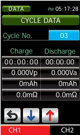
... It is possible to scroll through the data of other cycles with the INC or DEC key.
