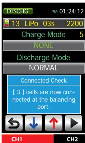
NiCd and NiMH batteries charge process starts as described below by way of example for a lithium battery after about 5 seconds. For lithium batteries and PB after few seconds the battery test, it is carried out a review of the number of cells connected batteries.
