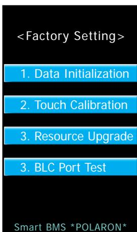
Press and hold the push button placed under the display and turn on the charger. After a short time, the display will appear as shown on the left.
