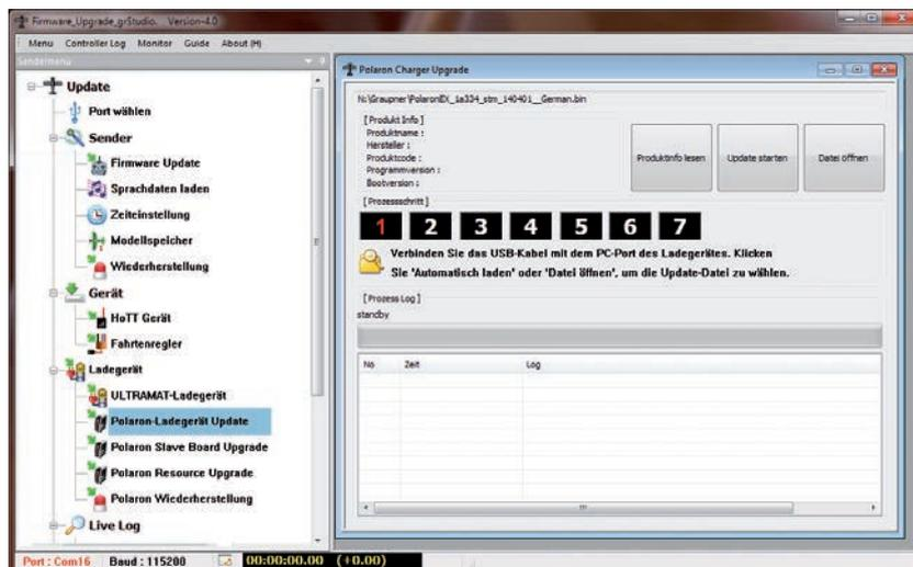
Click on the button "Open File" and select, in the Explorer window that appears, in the folder in which the previously downloaded and unzipped firmware files, ending with "... .bin", are located:
