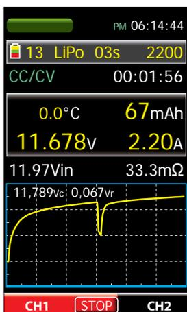
After the lapse of the aforementioned 5 seconds or if necessary, after a manual start, charge process is begun. Otherwise, an error message is shown.
