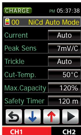
Add now the menu “PROFILE” key data concerning your batteries in this menu “CHARGE” with the corresponding charging parameters. To do this, choose the battery type and cell number matching the battery to charge. So If necessary, tap with your finger or the pen supplied in a lateral recess of the device to the “memory field”. In the blue area now select via the INC / DEC buttons at the bottom of the display the desired memory location 0 ... 19.
