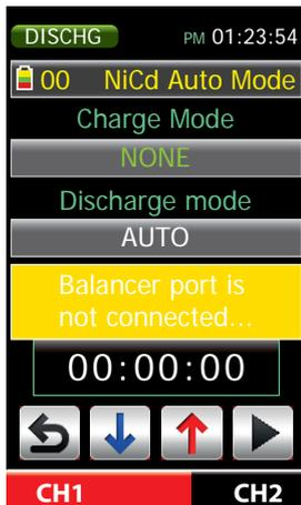
... One-tap the ENTER button on the bottom right of the display brings on the second display page of the „DISCHARGE“ menu.
