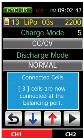
NiCd and NiMH batteries cycling process starts as described below by way of example for a lithium battery after about 5 seconds.
