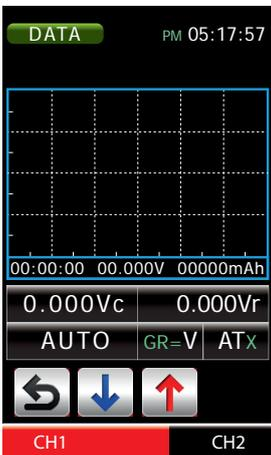
In this third display of "DATA" menu are shown graphically the charge/discharge data.
