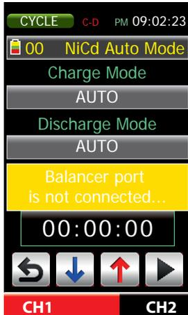
... Tap the ENTER button on the bottom right of the display brings on the second display page of the „CYCLE“ menu.
