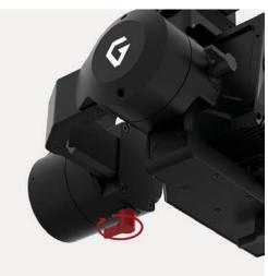
1. Loosen the thumb screw underneath 2. Tighten the thumb screw to lock the the roll bar, then gently slide the roll bar roll bar in position. left or right until roll axis remains level.
