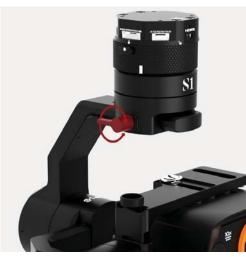
1. Loosen the thumb screw, then gently 2. Tighten the thumb screw to make slide the pan axis slider backward/ forward until it doesn't swing and stay at any given position when released.
