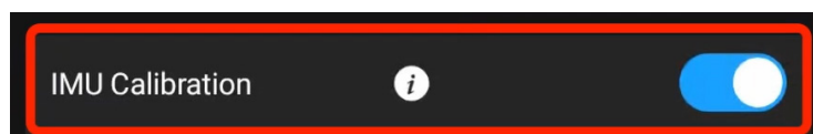
Figure: After IMU Calibration is enabled, Zenmuse L2 automatically calibrates the inertial navigation system based on the route, without the need for operators' intervention
