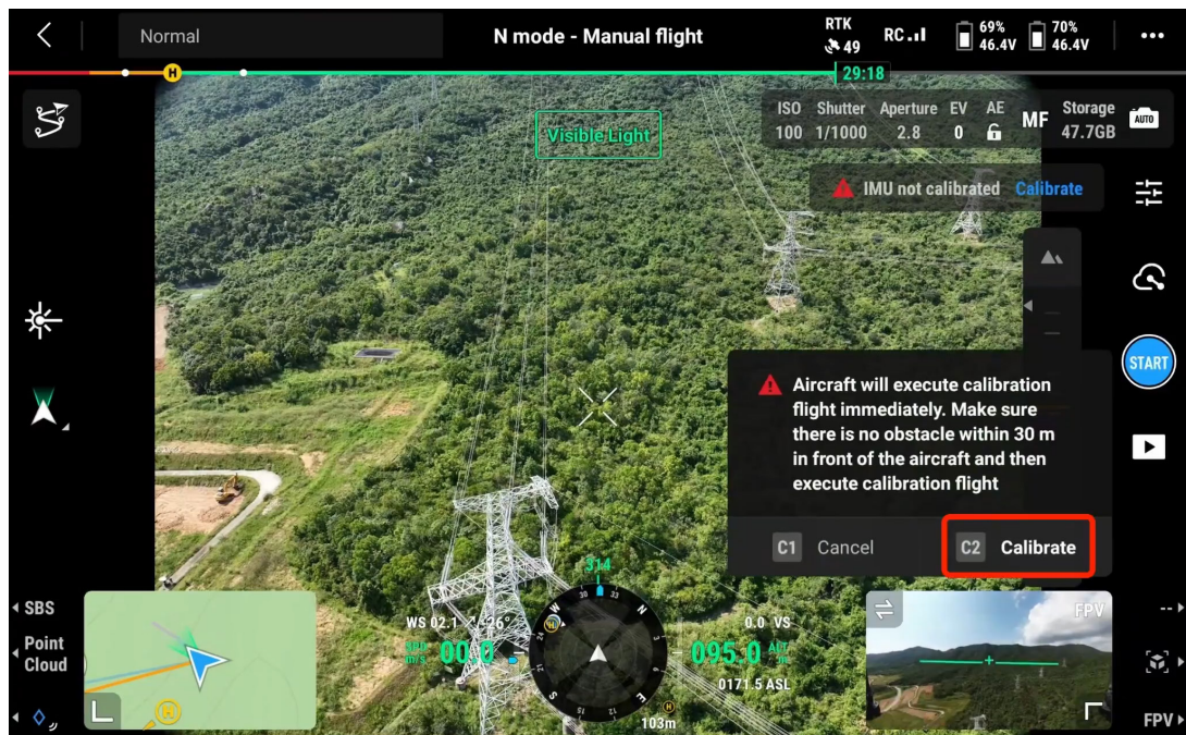
Figure: IMU calibration
