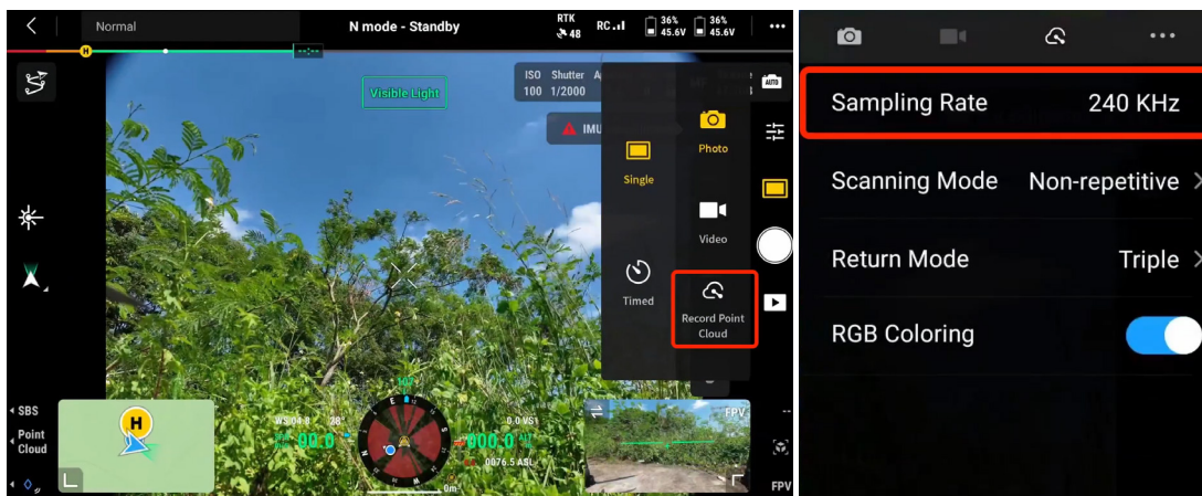
Figure: Enable point cloud recording
