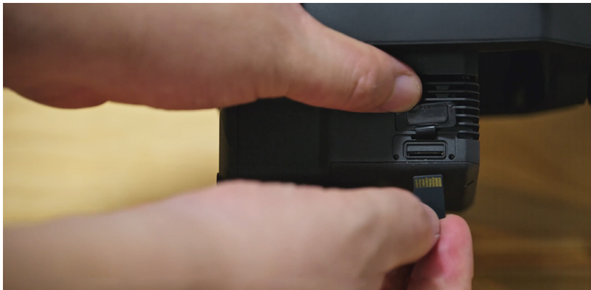
Figure: microSD card insertion
