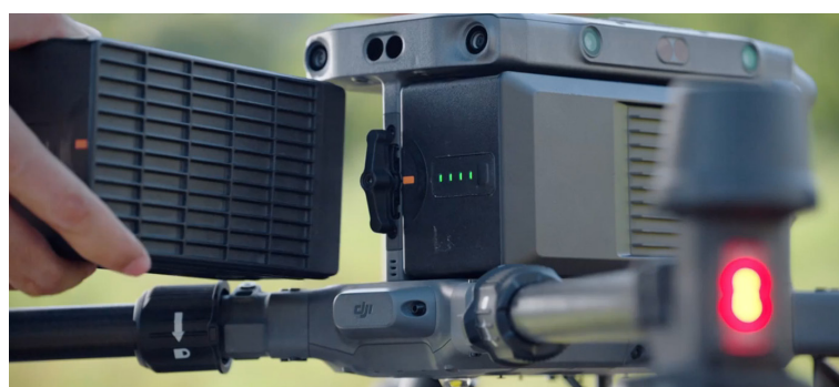
Figure: Battery hot-swapping
