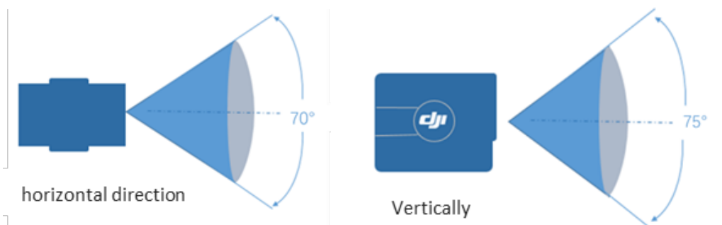
Figure: Scan angle in non-repetitive scanning mode
