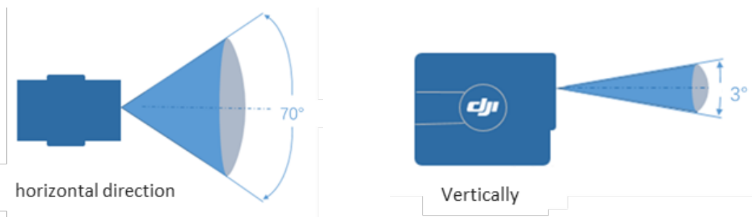
Figure: Scan angle in repetitive scanning mode
