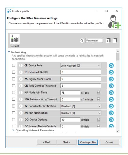
**Note** If you accessed the wizard from the **Configuration working mode**, the firmware settings should be already checked and selected with the ones configured in the XBee device.
