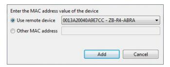
If no remote devices are discovered for the local device, you can enter the MAC address manually:
