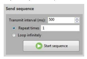
2. Click **Start sequence**. XCTU sends all frames in the **Send frames** list. Sent and received frames appear in the **Frame logs** area.
