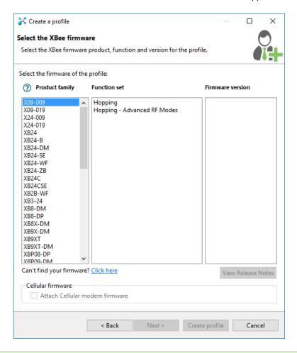
**Note** If you accessed the wizard from the **Configuration working mode**, the firmware should already be selected with the firmware that the XBee device is running.
