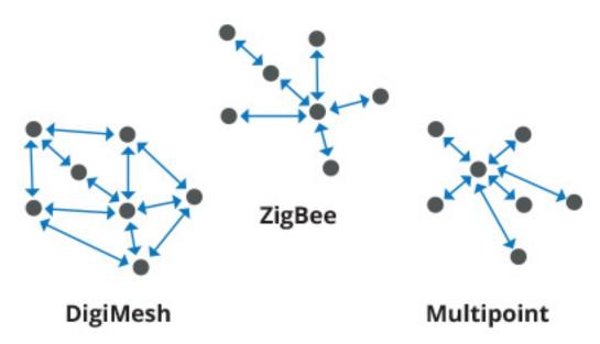
Not all XBee devices can run all listed communication protocols. The combination of XBee hardware and radio firmware determines the protocol that an XBee device can execute. For more information about the available XBee RF modules and the protocols they support, see XBee RF Family Comparison Matrix.
