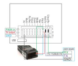
S.bus/Rx: connect to Rx2 for track function.
