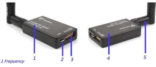
2 Micro-USB port 3 JST-GH 6-position port 4 LED indicator 5 2 dbi Antena
