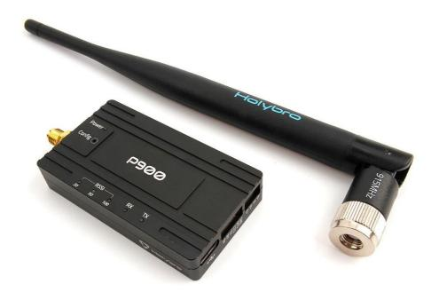
Holybro P900 Radio integrates microhard Pico Series P900 RF module which is capable of delivering high-performance wireless serial communications in robust and secure Mesh, Point to Point or Point to Multipoint topologies.
