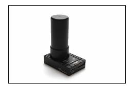
3) <u>H-RTK F9P Base (SKU12022) -</u> The board is the same as number 2 above, but it is equipped with a high-gain antenna. This model is best suited to use as base station. The search speed and positioning accuracy are the highest among the three models.
