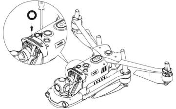
4. Power on the aircraft. If the connector cable is successfully connected, the gimbal will automatically rotate to perform a self-check.
