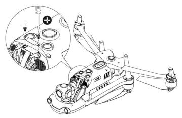
3. Insert a screw into a hole of the decorating part of the gimbal, and then screw it in with a T6 screwdriver until the screw is fixed but not tightened. For the other screw, repeat the same step. Fully tighten the two screws with a screwdriver.
