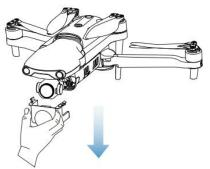
After you turn off the aircraft, you need to put the protective cover back on the gimbal to prevent damage.
