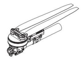
1. The entire power system has been assembled at the factory, and the power system can be taken out directly from the package, and installed on the frame of the plant protection aircraft according to the direction of rotation of the motor.
