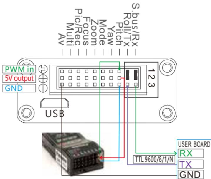
S.bus/Rx: connect to Rx2 for track function.
