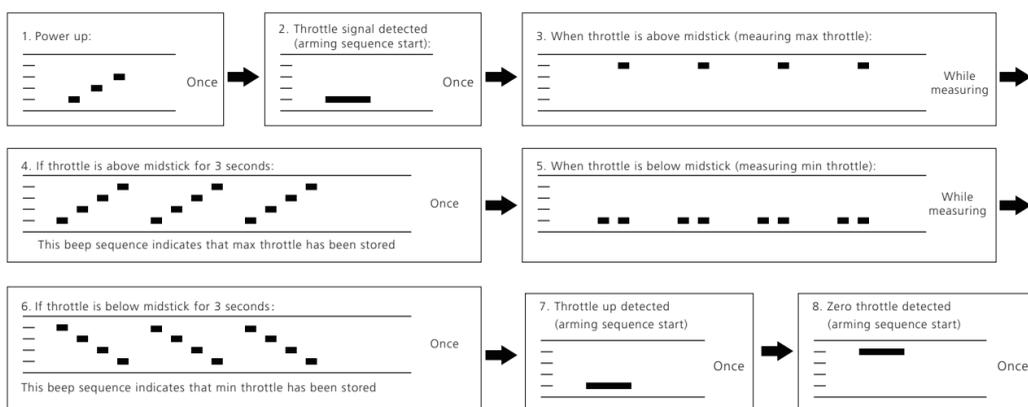
At this point throttle calibration values are stored. You may remove power from the ESC, or just continue running your ESC.
