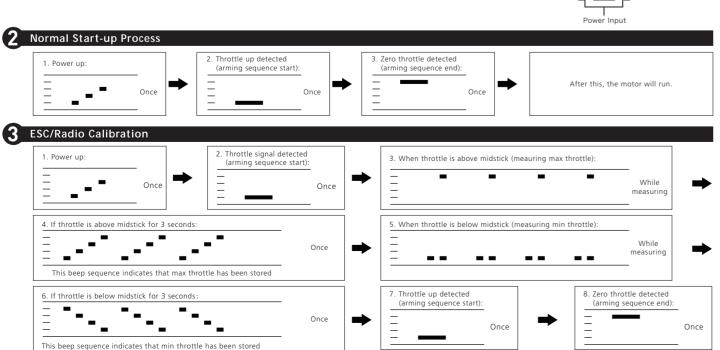
At this point throttle calibration values are stored. You may remove power from the ESC, or just continue running your ESC.
