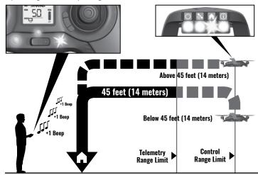
**Note:** If a control signal is reestablished between the transmitter and receiver along the return to home flight path, you may cancel Return to Home by pressing the *Air Brakes* button (see "Air Brakes" on page 11). Release the button to regain complete control of the model in **Film Mode**.
