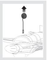
Make sure to reinstall the nose gear angled forward as shown.
