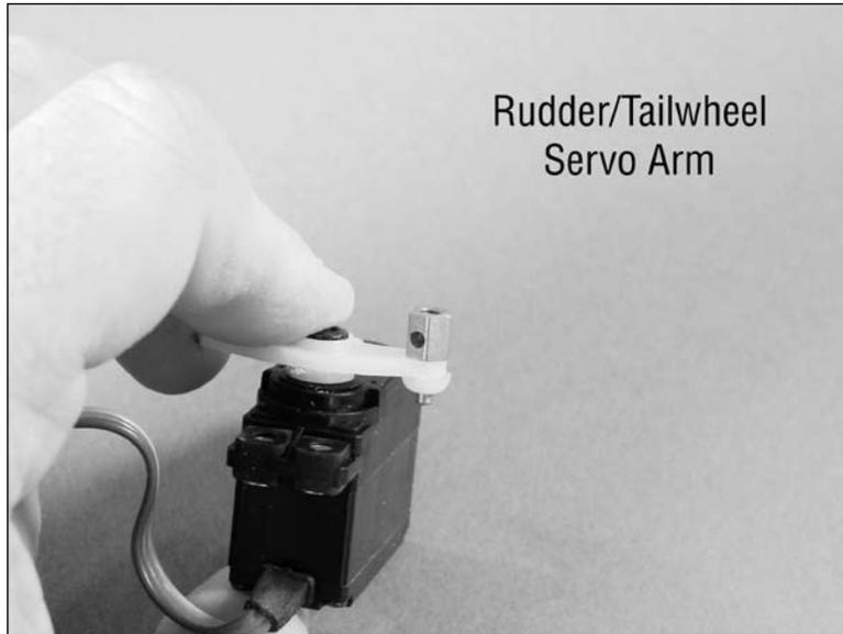
**Note:** If you are installing floats, prepare the rudder control horn as shown. The pushrod and brass connector will be on the same side of the servo horn.
