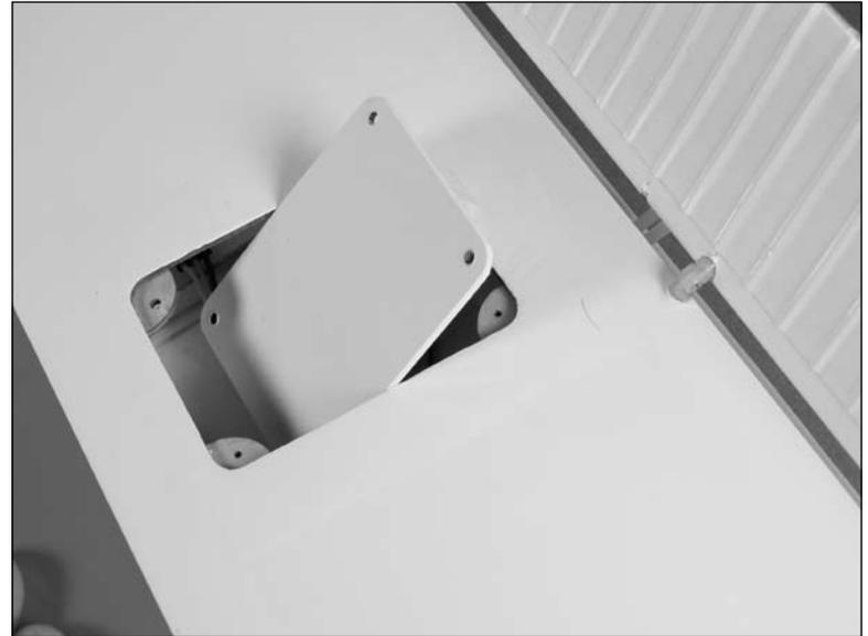
**Note:** *Do not* place or secure the flap servo cover in position before turning on the radio and checking the operation of the flap. Doing so could damage the flap control horn or quite possibly the flap servo. Check the length of the linkage as follows BEFORE installing the flap servo cover.
