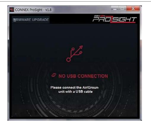
Connect the Micro USB Cable between the HD receiver micro USB port (1) and the computer USB port. The application's main screen opens.
