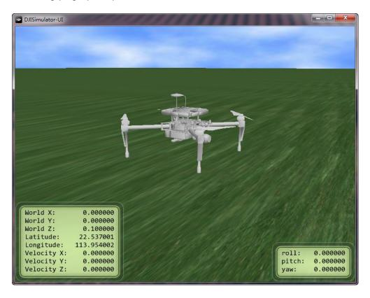
The user should be able to control the aircraft in the DJI PC Simulator by now. Otherwise, check the connection between the Matrice 100 and the computer. The DJI PC Simulator reflects the aircraft movements and behaviors in a virtual environment. Always run a simulation from the DJI PC Simulator for your application before apply the application in physical environment.
