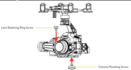
**Step2:** Mount the camera into the gimbal. Tighten the Camera Mounting Screw first then tighten the Lens Retaining Ring Screw.
