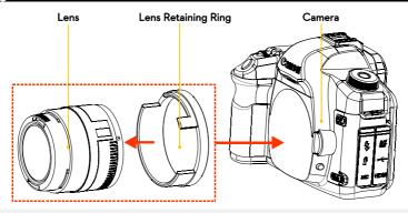
Step 1: Mount the lens on the retaining ring first, before mounting the lens to the camera.
