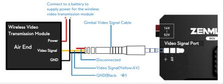
**Stepl:** Solder the Power/Video Signal/GND cables to a wireless video transmission module (Air End) respectively.
