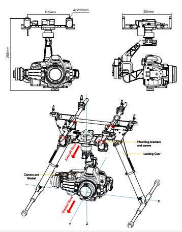
Step3: Attach the gimbal to the landing gear then tighten the thread locking screws.
