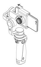
The system is balanced if the mobile phone remains level when released, balanced only by the gimbal.
